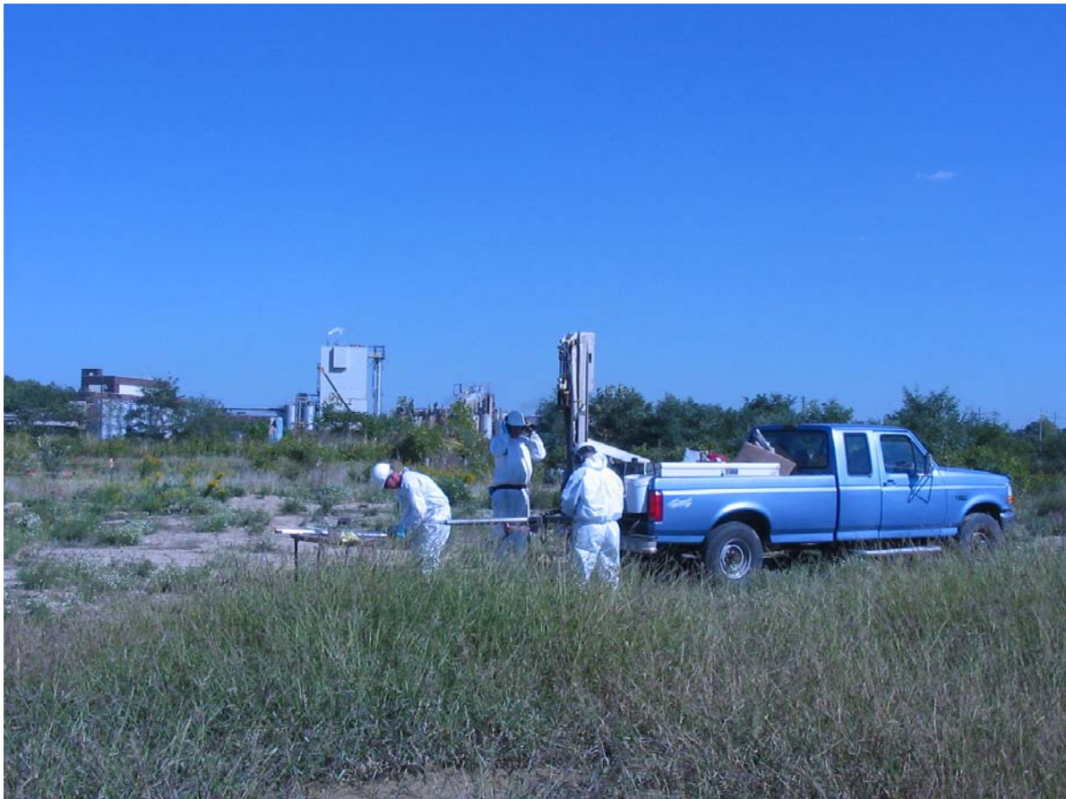
Figure 3-1. Earthprobe™ Sampling Rig Mounted on Truck
