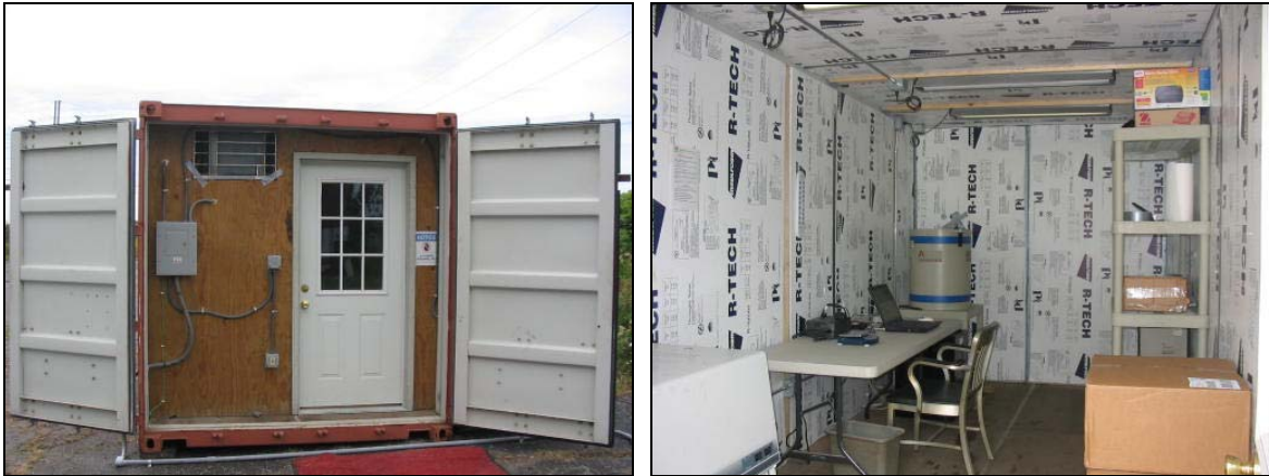
Figure 3-3. Exterior and Interior Photographs of Retrofitted Onsite Gamma Spectroscopy Laboratory
