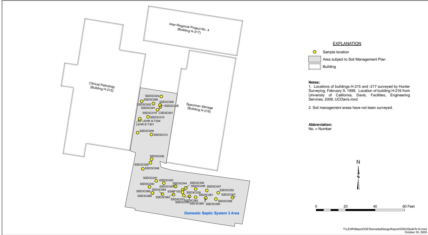
Attachment B Figure 2. Soil Sample Locations for the Domestic Septic System 3 Area (>4 to 10 Feet Below Ground Surface)
