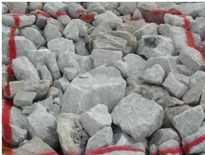
Photo 18. Cell cover rock test plot TP5; located on upper west side (2005 Inspection).
