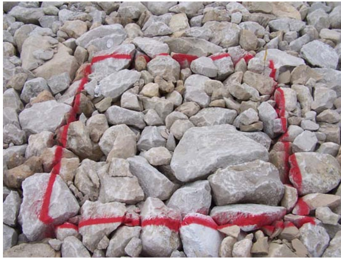
Photo 10. Cell cover rock test plot TP1; north edge of north facet (2005 Inspection).
