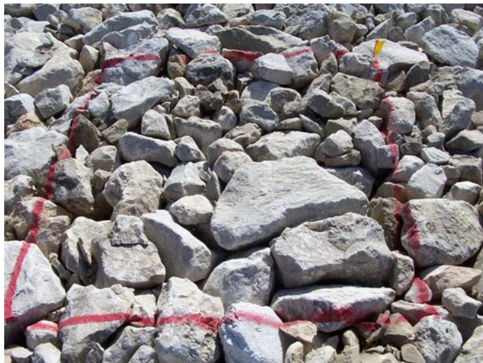
Photo 12. Cell cover rock test plot TP1; north edge of north facet (2007 Inspection).
