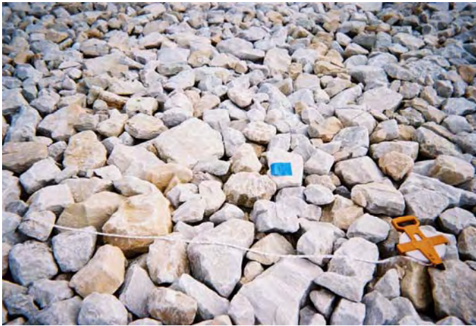
Photo 19. Cell cover rock est plot TP5; located on lower west side (2003 Inspection).
