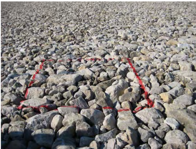
Photo 14. Cell cover rock test plot TP3; northeast ridgeline (2008 Inspection).
