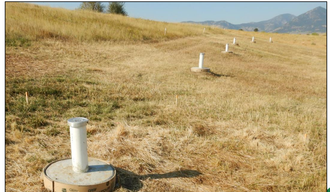
Piezometers west of SPPTS groundwater collection trench
