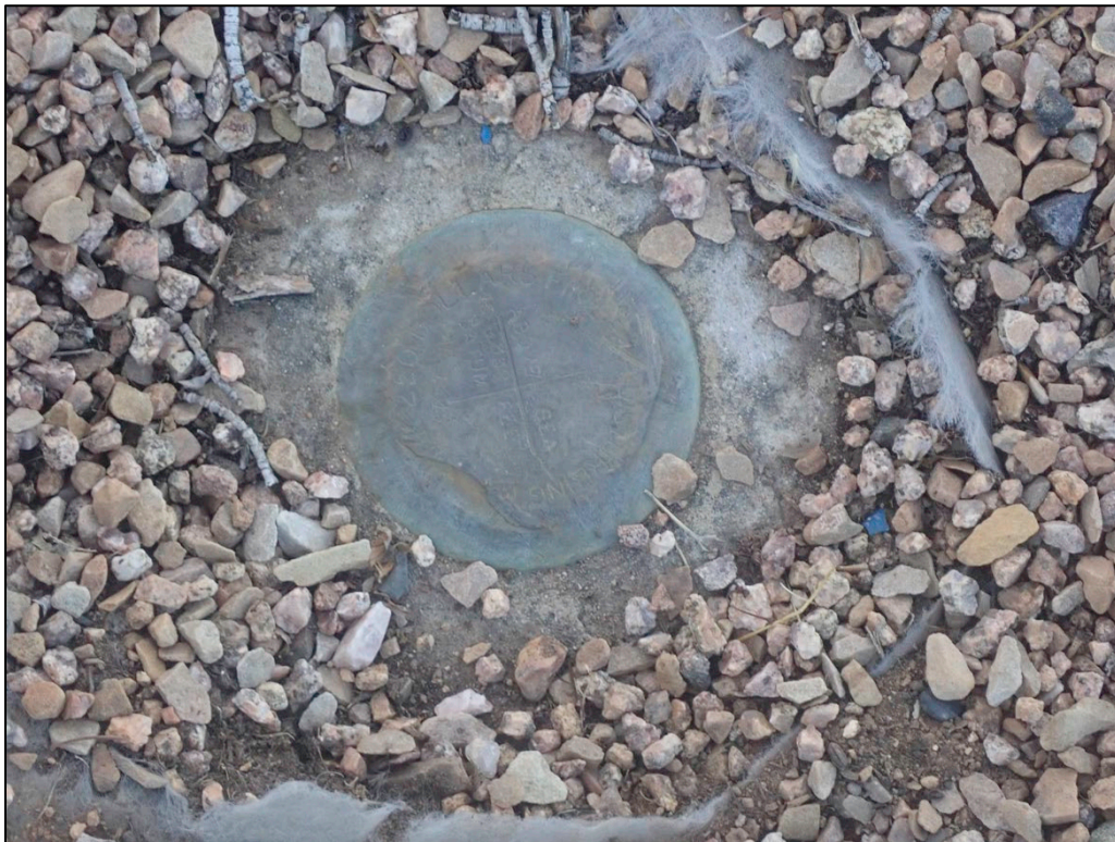
PL-1. National Geodetic Survey Monument
