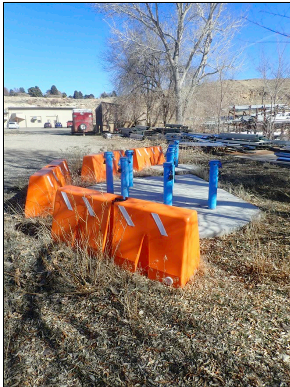
PL-5. Applied Studies and Technology Monitoring Well Gallery
