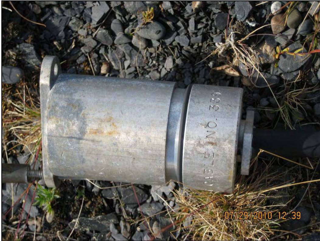
Photograph 19 – Closeup of thermistor cylinder found on pad near Test Hole Dog.
