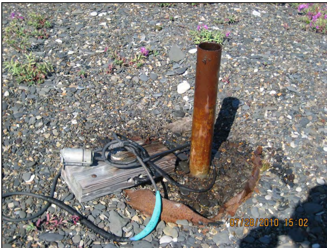
Photograph 10 – Test Hole Charlie with thermistor cable, block of wood, and cylinder on ground.
