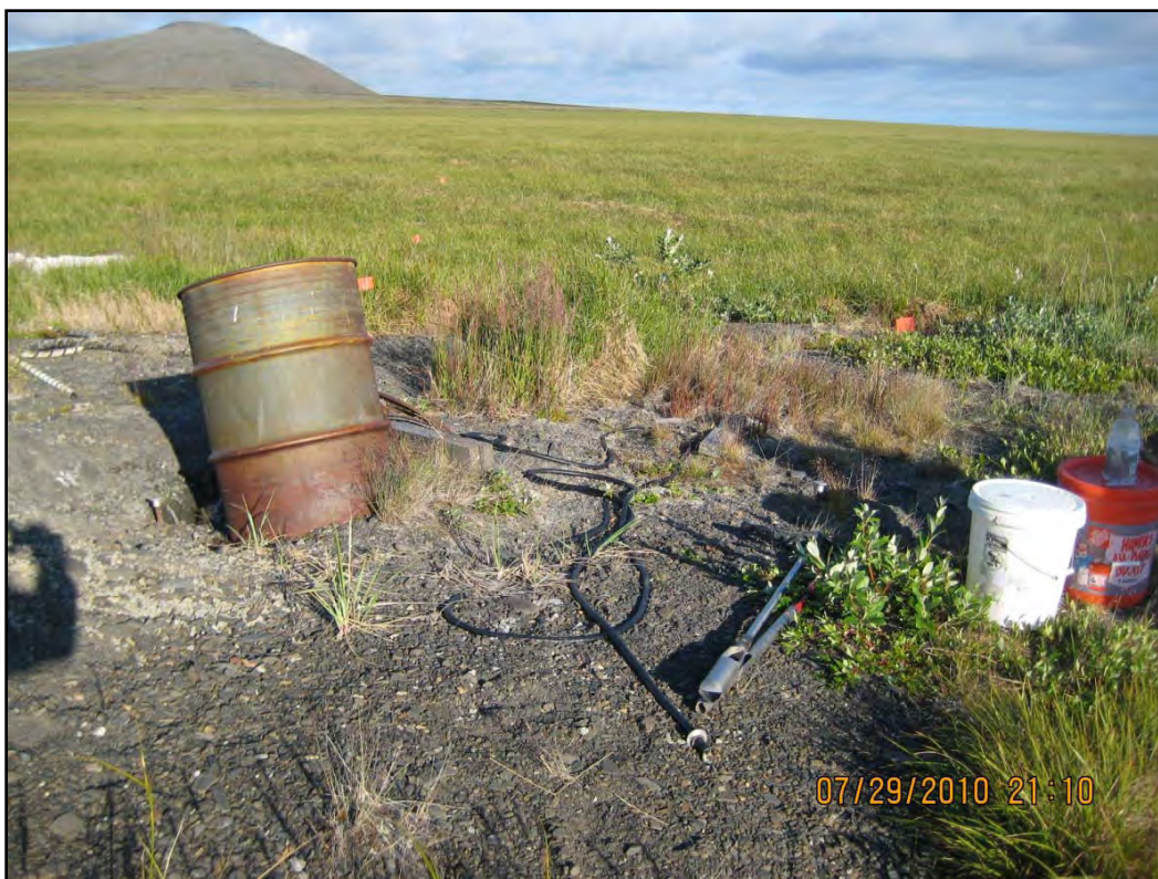
Photograph 7 – Test Hole Baker, thermistor cable, auger, decon water, and pin flags (View to NE).
