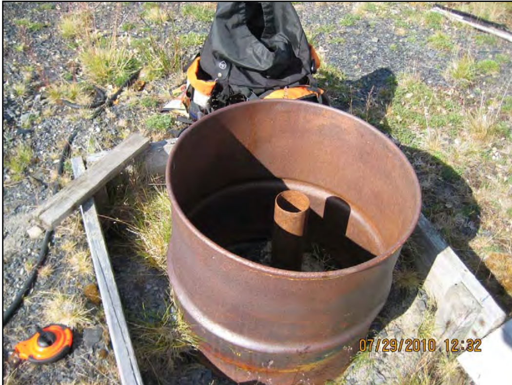
Photograph 17 – Test Hole Dog with steel drum protective casing and wood structure.
