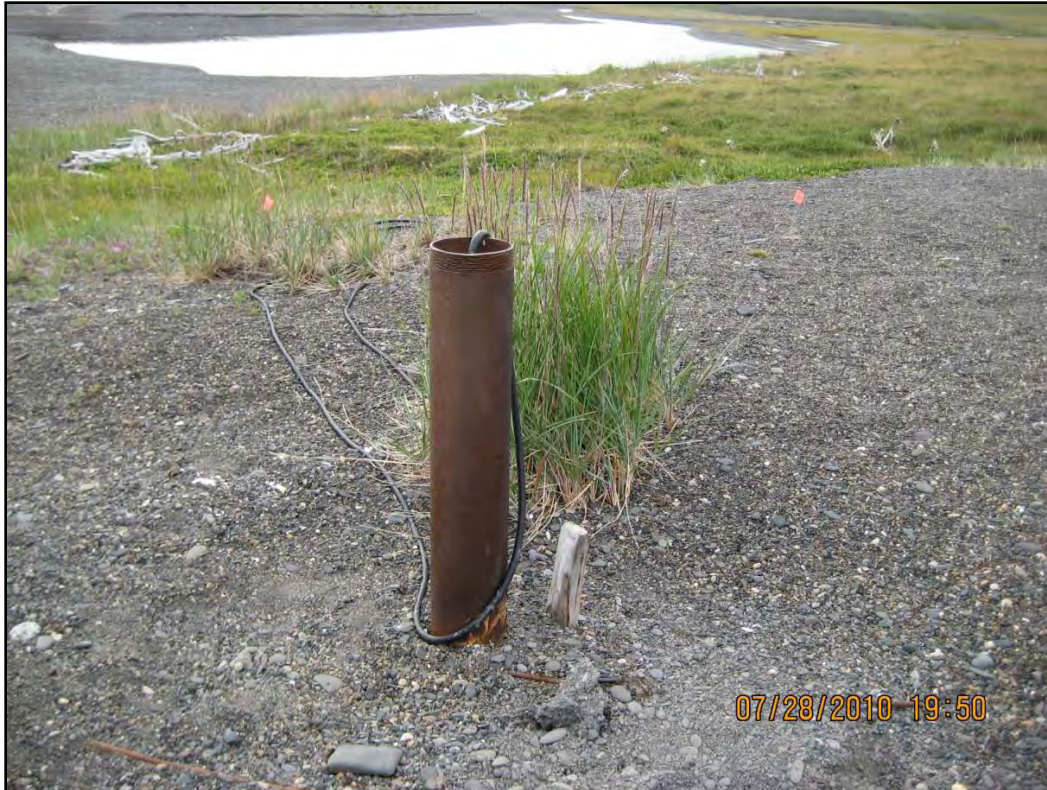
Photograph 3 - Test Hole Able and thermistor cable. Ogotoruk Creek in BG (View to W).
