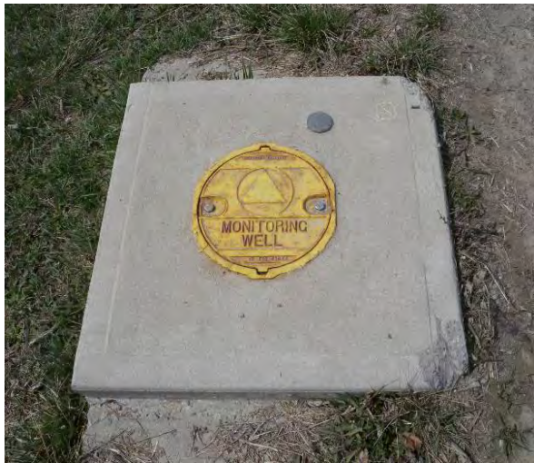
Figure 30. Parcel IC Well P033, in Good Repair and with a Permanent Identification Marker
