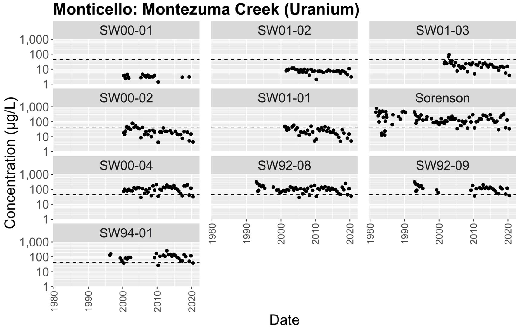
Figure 30. OU III Surface Water Uranium Concentration Trends
