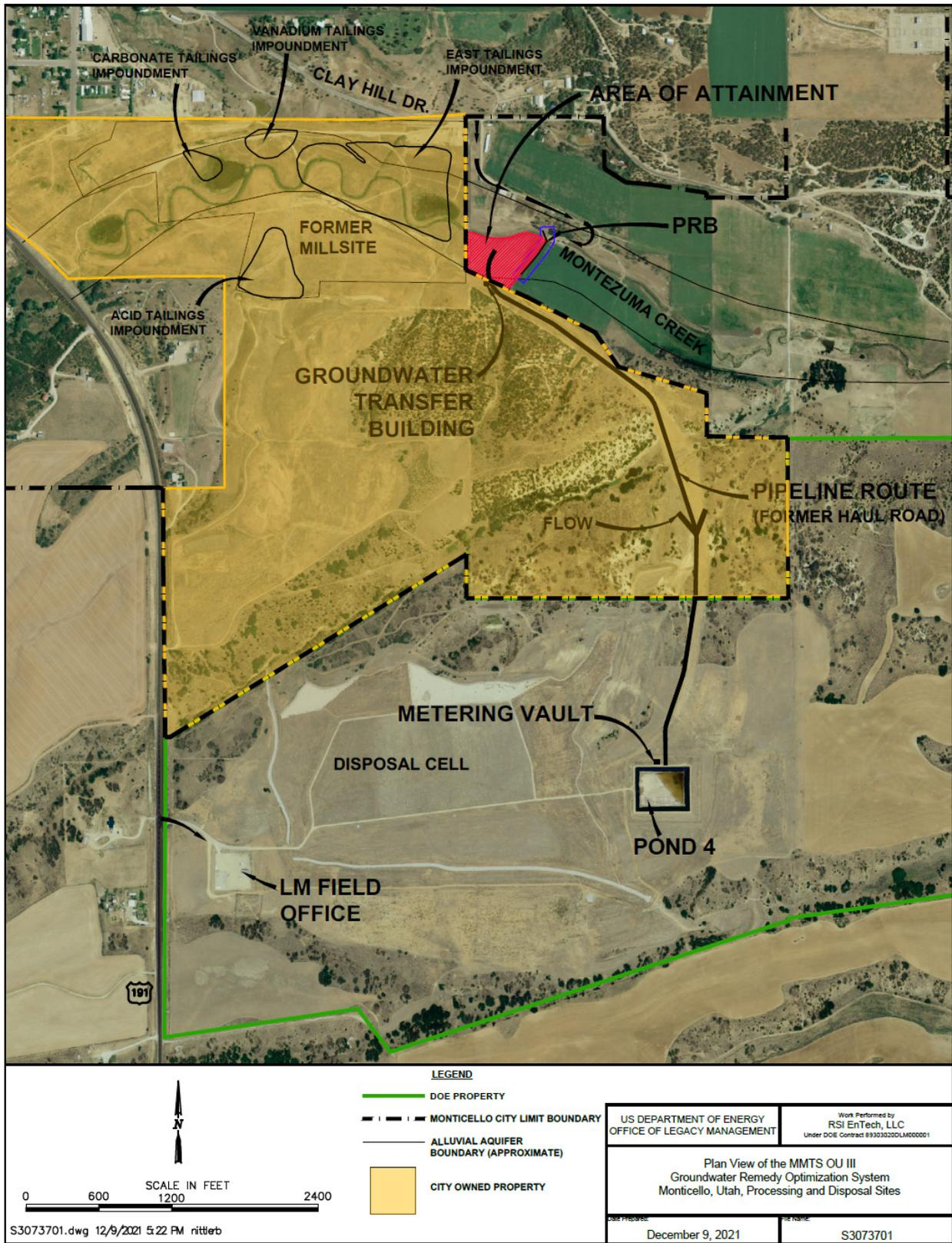
Figure 2. Monticello Mill Tailings Site Historical and Current Features
