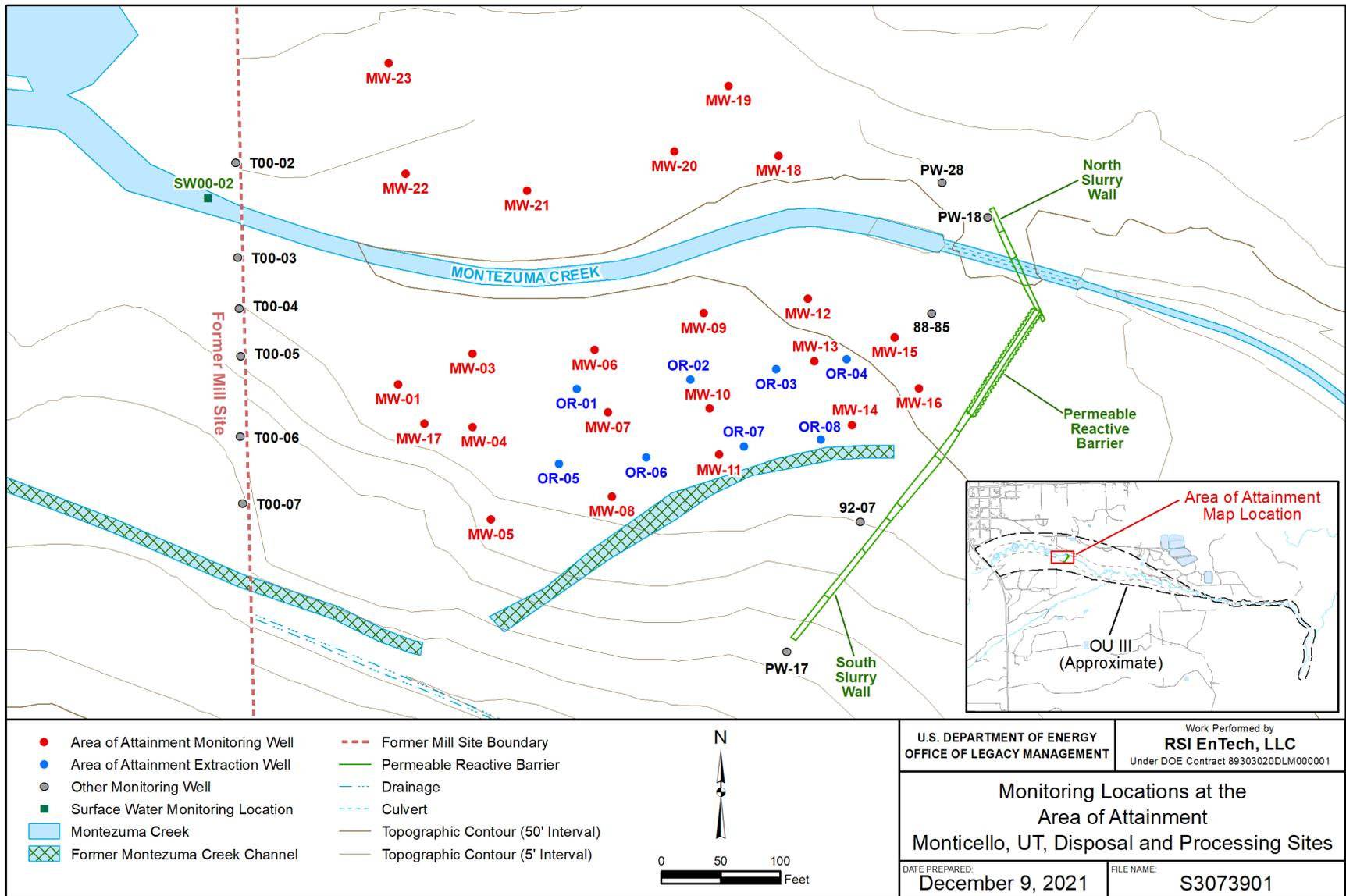
Figure 4. AOA Extraction and Monitoring Well Locations
