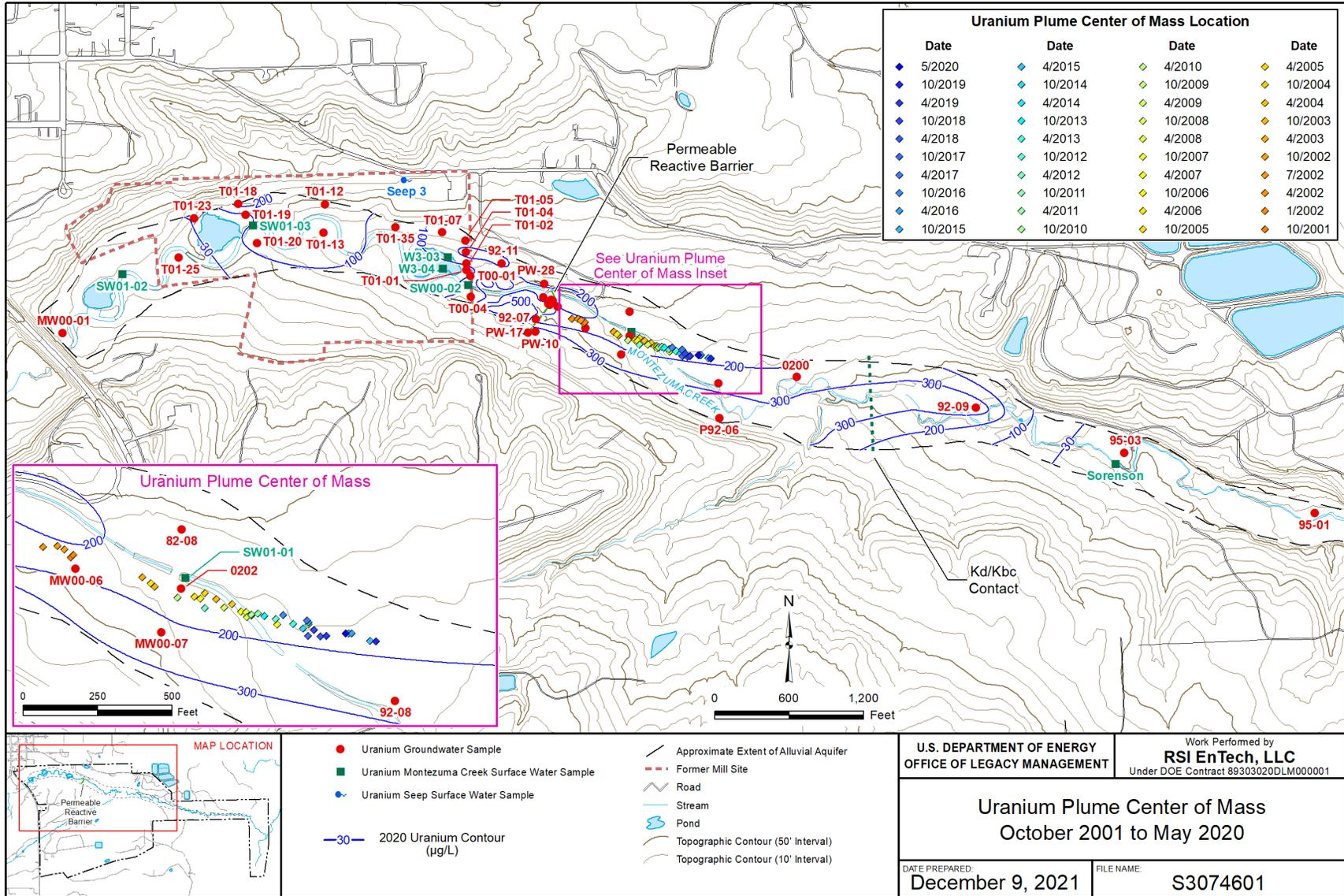
Figure 29. OU III Uranium Plume Center of Mass Temporal Locations
