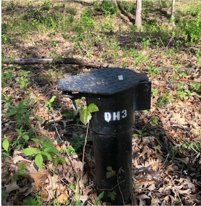
P11 - Monitoring Well DH03 at Red Gate Woods
