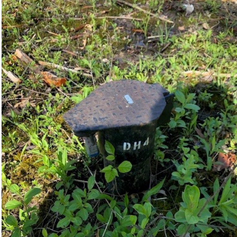
P12 - Monitoring Well DH04 at Red Gate Woods
