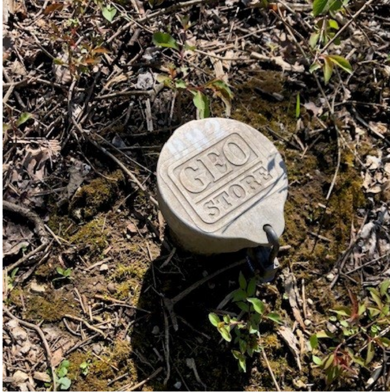
P01 - Monitoring Well BH02 at Plot M
