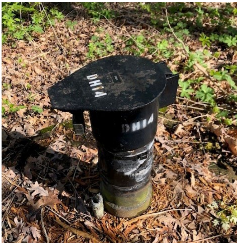
P15 – Monitoring Well DH14 at Red Gate Woods
